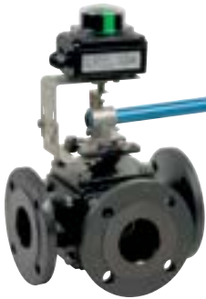
783 - Carbon steel - L port A216WCB body - PTFE seats - Full bore - PS: 16 bar - TS: -20°C/+150°C.
