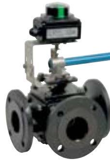
784 - Carbon steel - T port A216WCB body - PTFE seats - Full bore - PS: 16 bar - TS: -20°C/+150°C.
