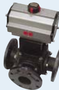
783 L-port / 784 T-port - Pneumatic actuated 3 way carbon steel ball valve A216WCB body - CF8 ball - TS: -20°C/+150°C.
